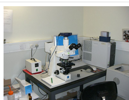
A modern microscope with a mercury bulb for fluorescence microscopy. The microscope has a digital camera, and is attached to a computer.
